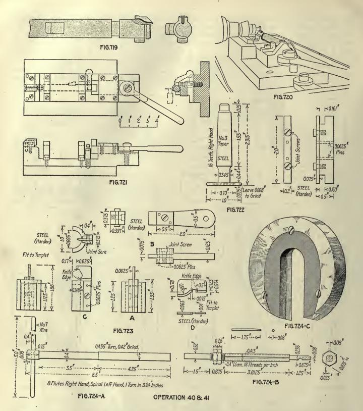
OPERATIONS 40 AND 41. HAND MILLING EJECTOR SLOT,
