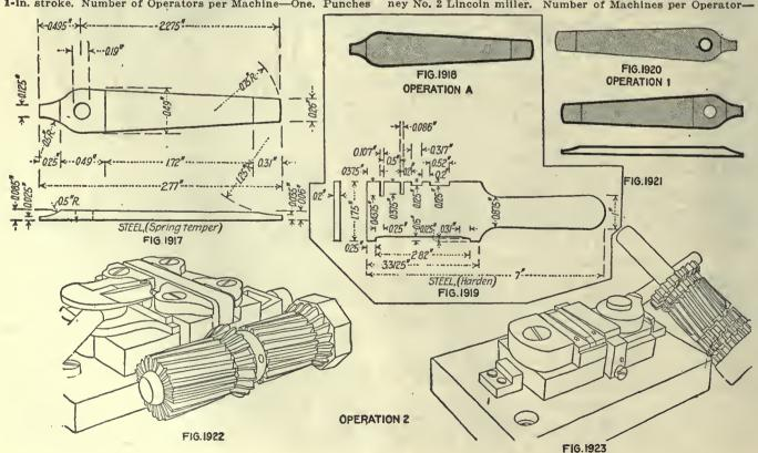
Four. Work-Holding Devices—Held by vise jaws, Fig. 1922 and 1923. Tool-Holding Devices—Standard arbor. Cutting Tools—Gang of milling cutters, Figs. 1922 and 1923. Number of Cuts—One. Cut Data—70 r.p.m.; §-in. feed. Coolant—Cutting oil, put on with brush. Average Life of Tool Between Grindings—5000 pieces. Gages—Fig. 1924, width, thickness and length. Production—45 pleces per hr.
