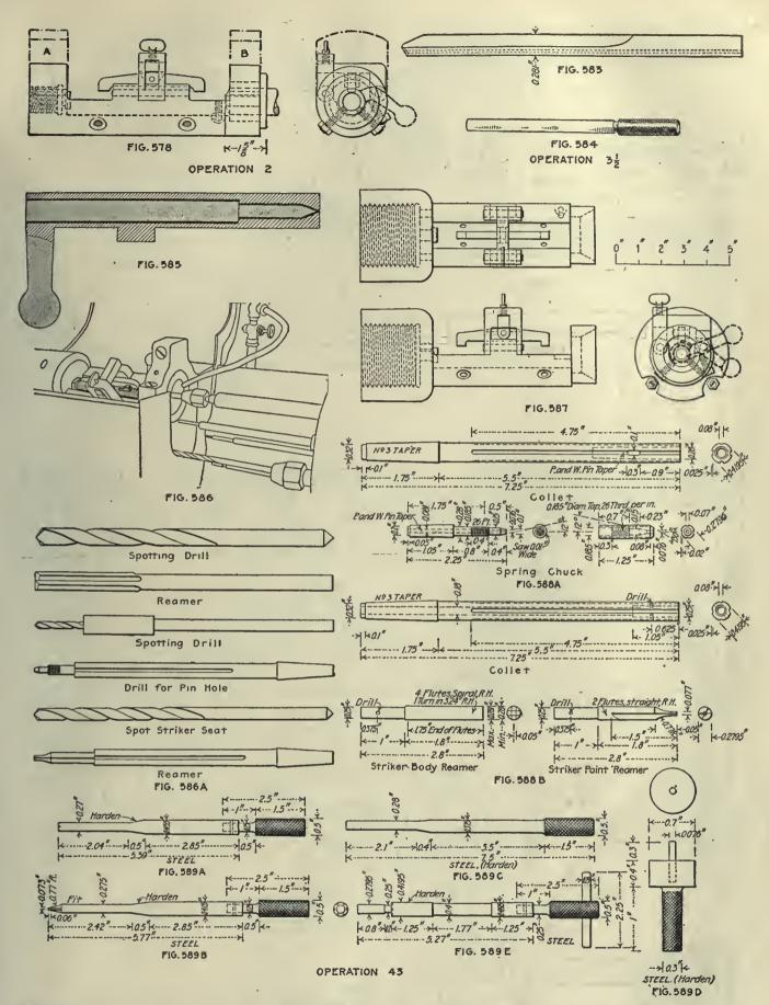
OPERATION 43. DRILLING AND SHAPING STRIKER SEAT Transformation—Fig. 585. Machine Used—Pratt & Whitney hand screw machine, 16-in., Fig. 586; machining diagram, Fig. 586-A. Number of Operators per Machine—One. Work-Holding Devices—Revolving fixture, Fig. 587. Tool-Holding Devices—Drills in turret of machine. Cutting Tools—Two drills, one countersink, one bottoming drill
