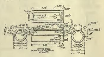
FIG. 157. DETAILS AND WORKING LIMITS OF THE FIXED BASE
