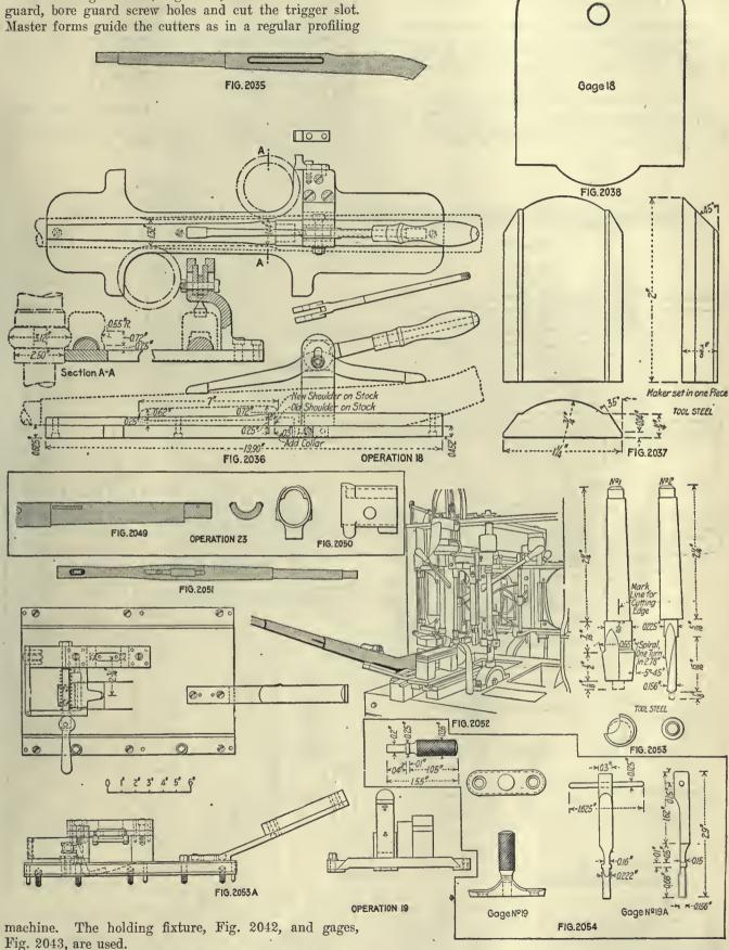
The hole and slot for the lower-band spring are made seat to exact size and shape. Rounding the edge under in the machine shown in Figs. 2045 and 2045-A. The the upper band is a hand operation with a spoke shave.
