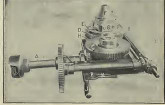
FIG. 98. RELIEVING ATTACHMENT FOR ROLL GROOVING
