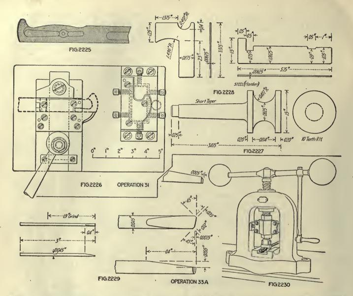
shank. Dies and Die Hoiders-Fixture bolted to bed of press; stamps are set in die. Production-350 pieces per hr. Note-Dies stamp "U. S." on one side and "ball and flame" on the other.
