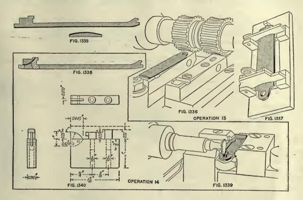
OPERATION 91/2. FILING LUGS TO MATCH PROFILING AND MILLING CUTS
