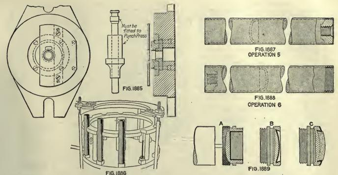
OPERATION 3. SWAGING AND ASSEMBLING LEATHER Transformation—Fig. 1889-C. Machine Used—Old 10-in. Prentice lathe. Number of Operators per Machine—One. Work-Holding Devices—Draw-in chuck. Tool-Holding Devices—Crossfeed. Cutting Tools—Swaging or spinning tool. Number of Cuts—One. Cut Data—250 r.p.m.; hand feed. Production—350 pieces per hr.
