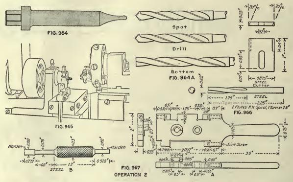
OPERATION 2. SQUARING AND DRILLING REAR END IN HAND SCREW MACHINE
