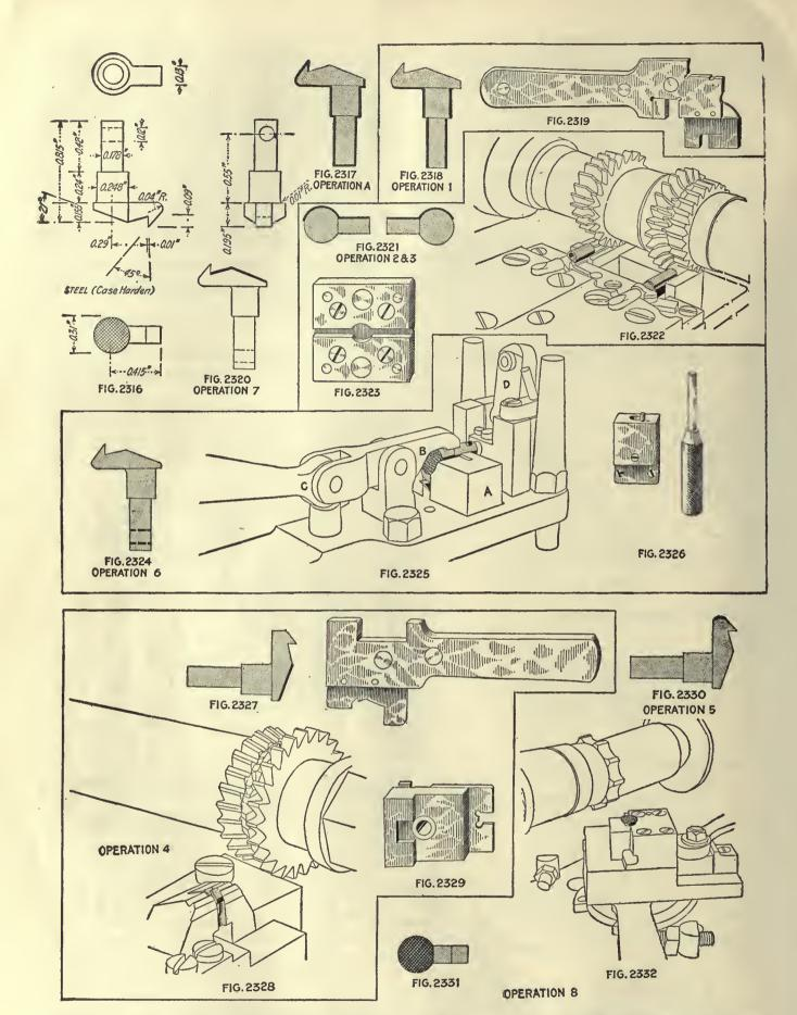
Holding Devices—Drill jig. Fig. 2325; holds work in V-block, by finger B and cam C; drill bushing in surveying leaf D. Tool-Holding Devices—Drill chuck. Cutting Toois—Twist drill. Number of Cuts—One. Cut Data—750 r.p.m.; hand feed. Coolant—Cutting oii, 15-in. stream. Average Life of Tool Between Grindings—500 pieces per grind. Gages—Fig. 2326, diameter of hole and location by using block. Production—125 pieces per hr.
