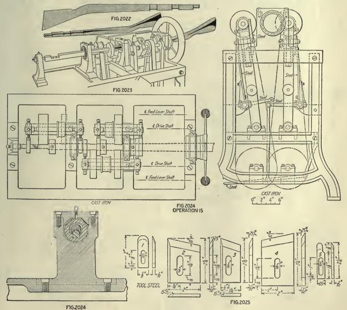
The modified Blanchard type of lathe referred to for finish cutting for the bands is fitted with cams for guiding the inscrted tooth circular cutters instead of the continuous master form of the stock turning machine.
