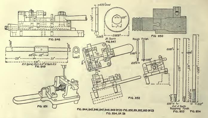
OPERATION 25. REAMING HOLE FOR SLEEVE LOCK, BURRING SAFETY-LOCK SPINDLE HOLE AND COUN-TERSINKING SLEEVE-LOCK PIN HOLE, ETC.
