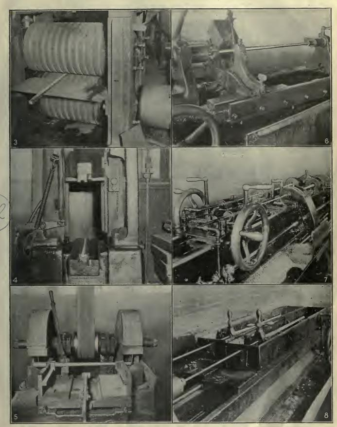
FIGS. 3 TO 8. SPECIALIZED OPERATIONS ARE FREQUENT IN MAKING THE SPRINGFIELD 1903 RIFLE BARREL Fig 3—Rolling barrels. Fig. 4—Hammer for straightening barrels. Fig. 5—Sawing barrels to rough length. Fig. 6—Turning outside of barrels. Fig. 7—Drilling holes in barrels Fig. 8—Reaming holes in barrels
