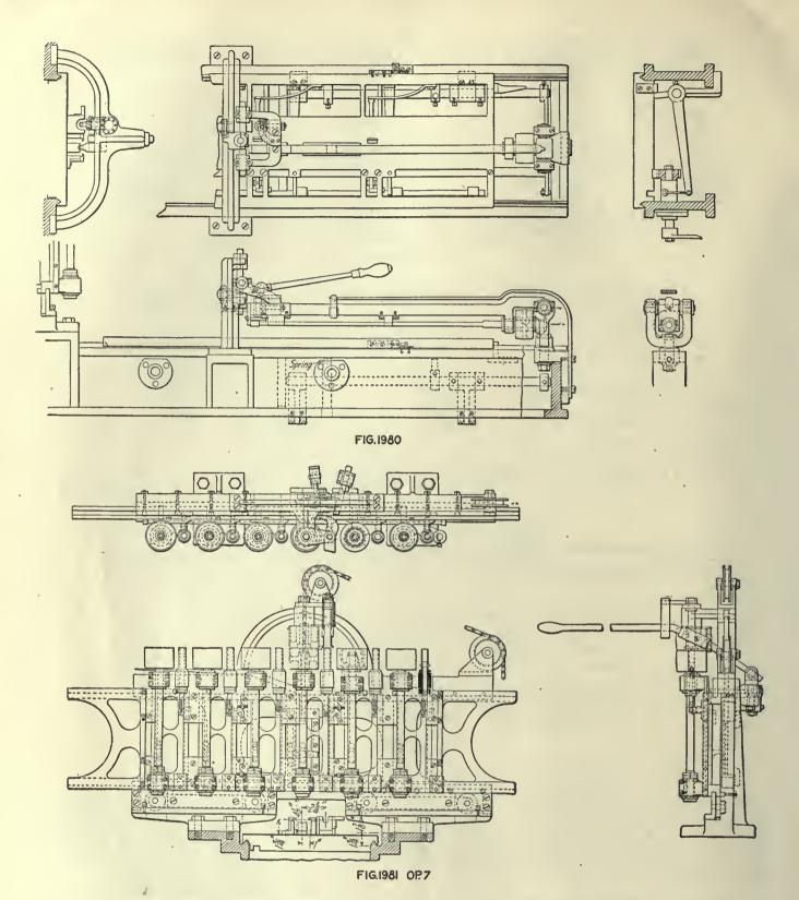
are fed in from opposite directions by means of a foot treadle. As the treadle is released, the heads recede; and as the lever is raised to release the work, the machine is stopped. One head carries two wood bits, which feed in about 0.3 in.; the other head carries a triangular-point center drill, which goes in just far enough to make a good center. The size and position of the driver-plate holes are gaged with the gages shown in Fig. 1956.
