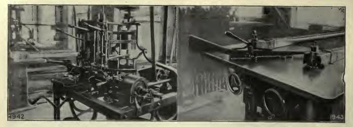
FIG. 1942. BEDDING AND DRILLING MACHINE
