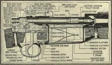
SYNOPSIS—Owing to the fact that the Springfield rifle, model 1903, cannot be produced in sufficient quantities, the Government has decided to adopt a modification of the English Enfield rifle, chambered for our regular cartridges. This article shows the rifle and its mechanism and also describes the action.
