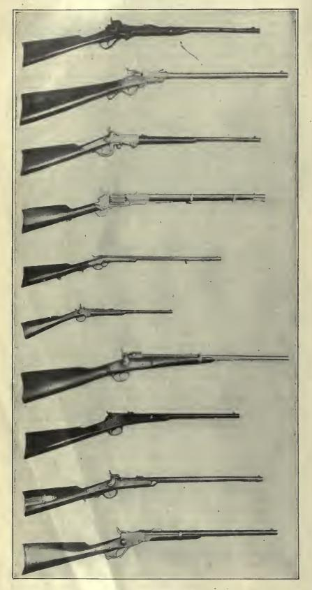
F1G. 29. SHARP'S CARBINE Patented Sept. 12, 1848, and Oct. 5, 1852; lever-action vertical sliding block; first ones used percussion caps and paper cartridges; cal. 50 and 52; length of barrel, 22 in.; total length, 39 in.; weight, 8 lb.; 80,512 purchased during Civil War
