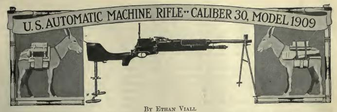
SYNOPSIS—This type of automatic rifle is air-cooled, but the radiating surface is not covered as in the Lewis gun. The feeding strips also differ from most others, which as a rule use belts. Sufficient details are given to insure a clear understanding of the mechanical action.
