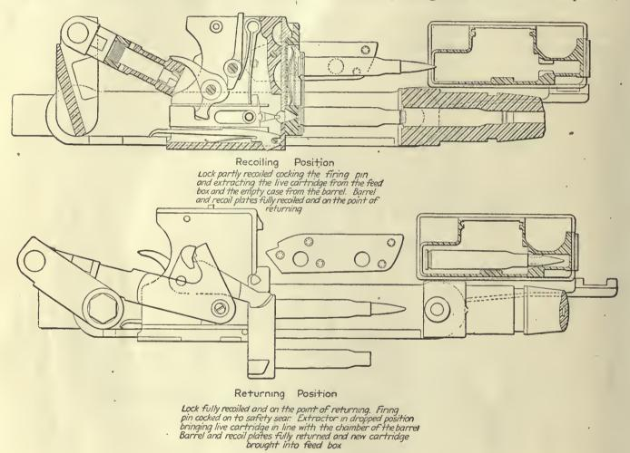
FIG. 5. THE ACTION IN RECOILING AND RETURNING POSITIONS
