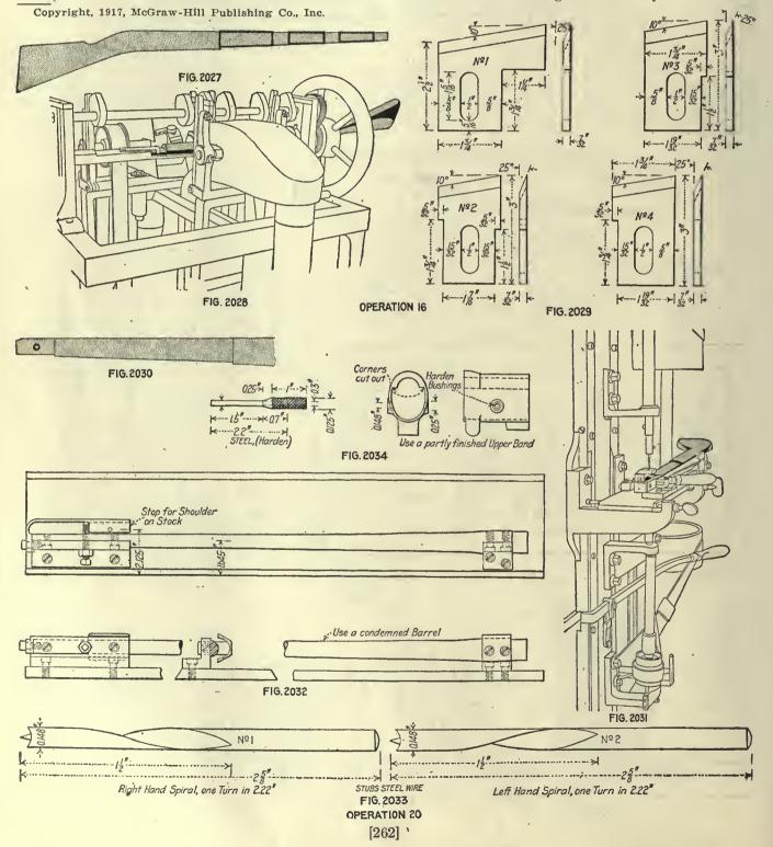
to give a good grip for the left hand. These grooves are cut in the wood shaper, Fig. 1943, using the work holder and form, Fig. 2036.
