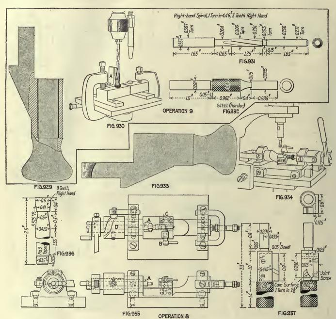
OPERATION 9. COUNTERBORING, FIRING-PIN BODY SIZE
