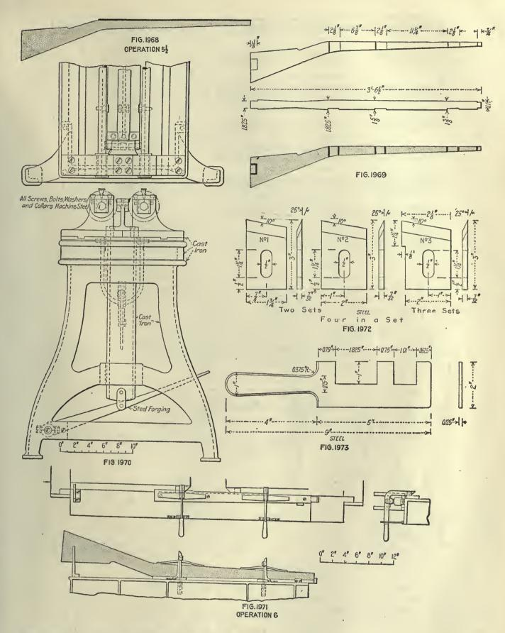
feeds toward butt; second cutter begins when first has fed along 6 in., the total cut being about 18½ in. Cut Data—Work turns about 50 r.p.m., cutters about 5000 r.p.m. Average Life of Tool Between Grindings—Stoned every 8 hr. Gages—Fig. 1963. Production—300 in 8 hr. for three machines. Note—One operator runs one lathe on this work and two on butts.
