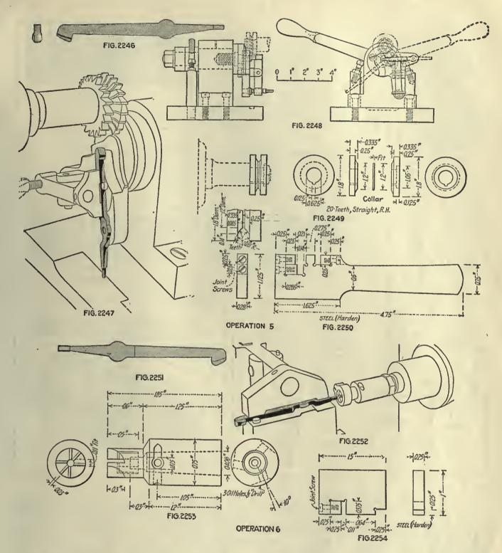
OPERATIONS BB AND CC. REMOVING BURRS LEFT BY OPERATIONS 3 AND 4
