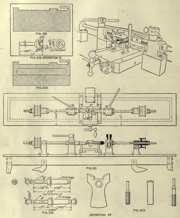
OPERATION 21. FILING MOVABLE BASE SEAT AND PIVOT Transformation—Fig. 218. Number of Operators—One. Description of Operation—Burring stud and filing base seat. Apparatus and Equipment Used—Hand hollow mili and also hollow cone file, Fig. 219; 6-in, piliar file. Gages—Straightedge. Production—25 per hr.
