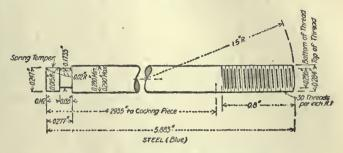
FIG. 881. DETAILS OF FIRING-PIN ROD
