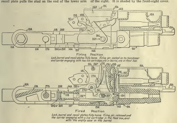
FIG. 4. THE ACTION IN FIRING AND FIRED POSITIONS
