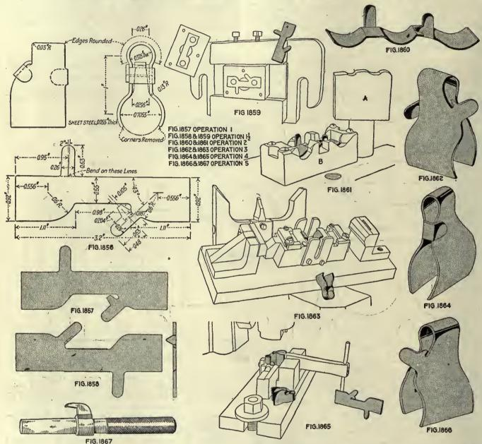
wood is used for the stock. Two of these clips are used on each guard, being fitted into recesses that prevent the interference of the hand guard and the barrel. They are made in a punch press with a simple bending die.
