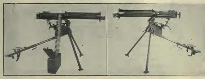
FIGS. 1 AND 2. OPPOSITE VIEWS OF VICKERS MACHINE GUN AND TRIPOD
