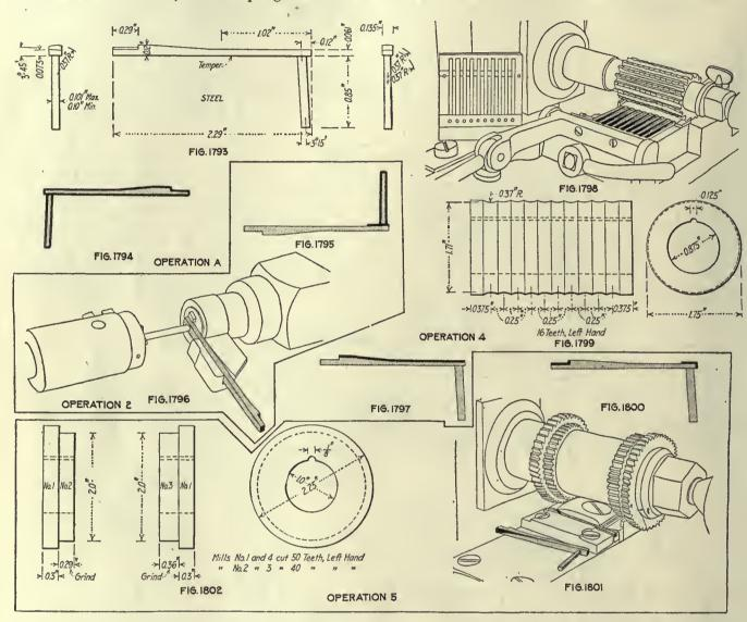
chined all over. It is then necessary to "set" the spring, and an ingenious little bench fixture is used for this purpose.
