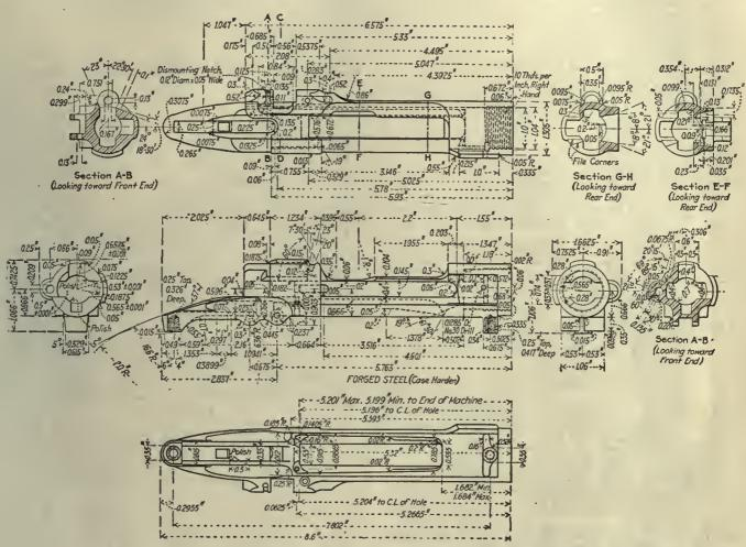
FIG. 251. DETAILS AND WORKING LIMITS OF SPRINGFIELD MODEL 1903 RIFLE RECEIVER
