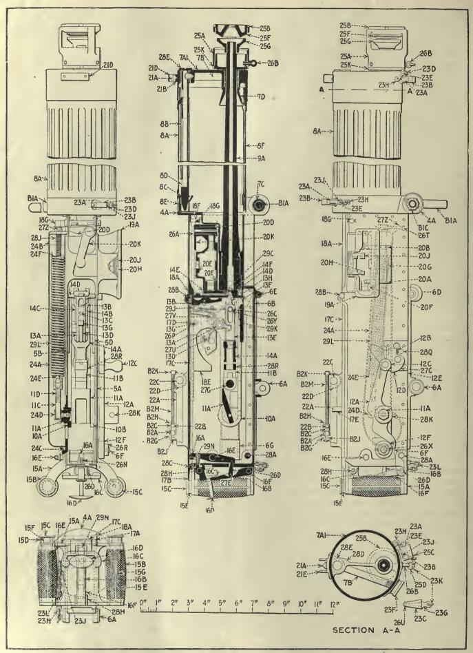
· FIG. 3. GENERAL ARRANGEMENTS AND SECTIONAL VIEW OF GUN
