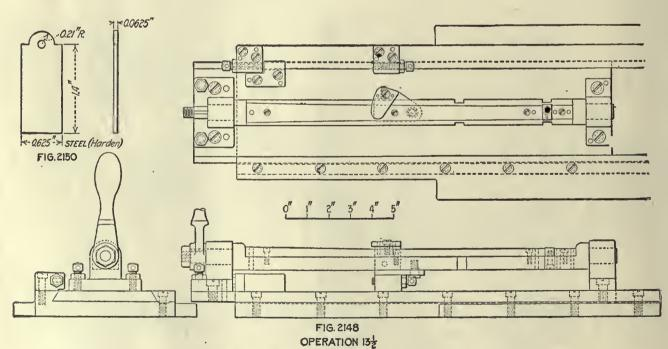
Average Life of Tool Between Grindings—500 to 700 pieces. Gages—Fig. 2139. Production—1210 per 8-hr. day. Note—Two pieces are turned at once; clip shown on work is to prevent spring and chatter during cut.
