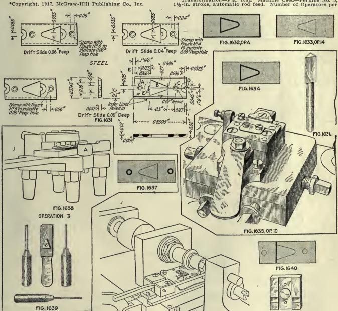
OPERATIONS ON THE DRIFT SLIDE, 0.05 PEEP Operation
