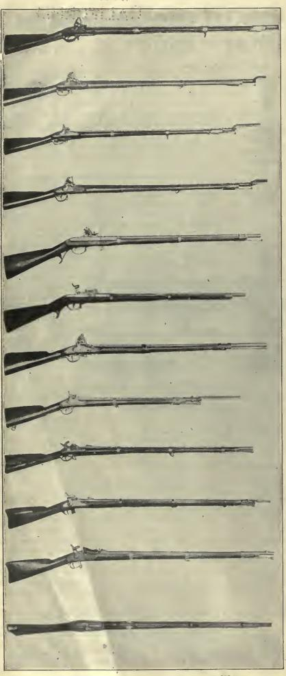
FIG. 3. UNITED STATES MUSKET, 1803 Fig. 3. UNITED STATES MUSKET, 1803 Flintlock; closely resembles French Charleville musket of 1763; made practically as in 1795 and following years at Springfield, Mass.; 71 cal.; diameter of breech, 2 % ln.; diameter of muzzie, % ln.; length of barrel, 42 ln. (barrel of 1809 musket was 45 ln. long); entire length, 56½ in.; weight complete, 10 lb. 7 oz.; without bayonet, 9 lb. 11 oz.; made at Springfield
