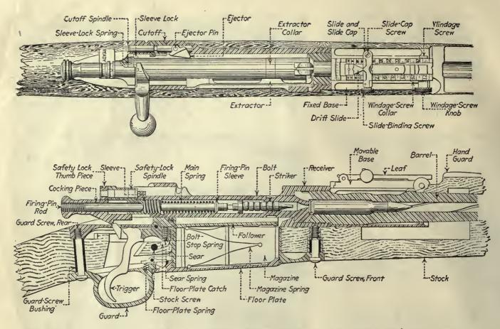
FIG. 26. SECTIONAL VIEW, BOLT AND MAGAZINE MECHANISM, U. S. MAGAZINE RIFLE, MODEL 1903
