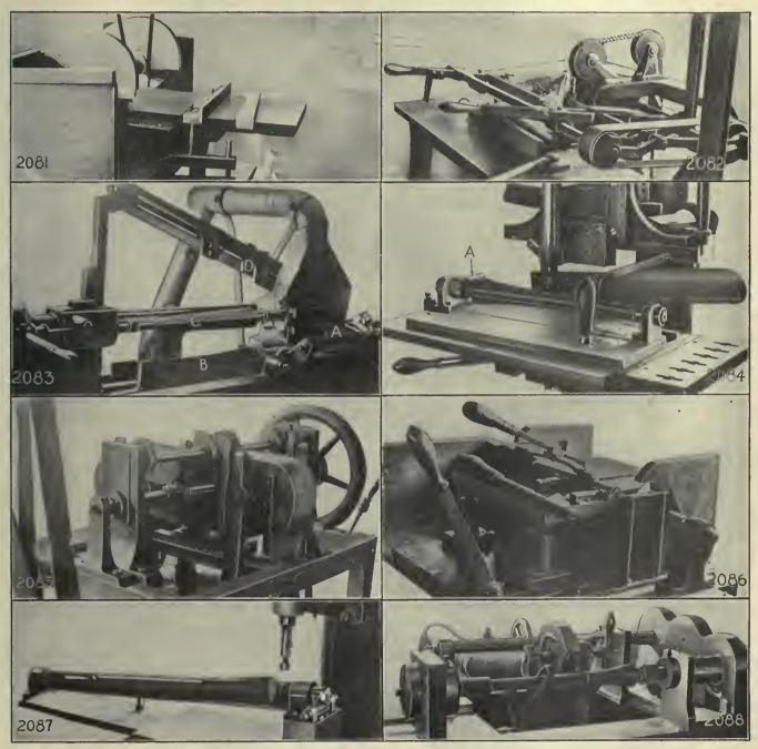
FIGS. 2081 TO 2088. VARIOUS OPERATIONS ON THE HAND GUARD Fig. 2081—Cutting to length for machinery. Fig. 2082—Grooving for barrel—second cut. Fig. 2083—Turning to remove stock. Fig. 2084—Cutting to match stock for width. Fig. 2085—Turning between bands. Fig. 2086—Cutting to finish length. Fig. 2087—Cutting clearance for windage screw. Fig. 2088—Finish-turning rear end
