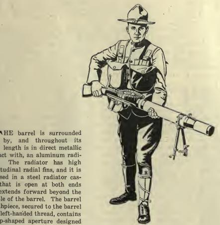
by, and throughout its length is in direct metallic contact with, an aluminum radiator. The radiator has high longitudinal radial fins, and it is inclosed in a steel radiator casing that is open at both ends and extends forward beyond the muzzle of the barrel. The barrel mouthpiece, secured to the barrel by a left-handed thread, contains a cup-shaped aperture designed
