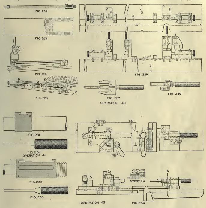
OPERATION 40. ASSEMBLING FRONT STUD AND FIXED BASE ON BARREL
