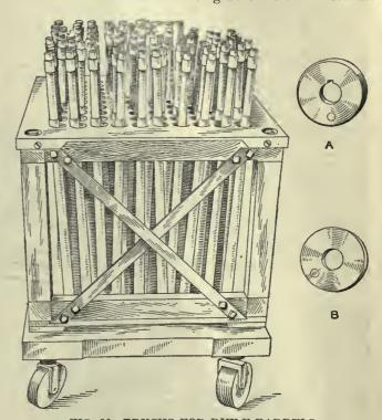
FIG. 96. TRUCKS FOR RIFLE BARRELS From the time the barrels are turned they are handled in special trucks, as shown in Fig. 96, holding 100 barrels each. These trucks are easily rolled from one machine to another and prevent damage to the barrels. After the thread is milled on the butt end for the receiver, the muzzle end is always placed down, so as to protect the thread.
