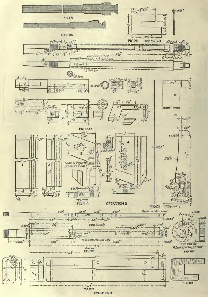
Holding Devices—Fig. 2105. Tool-Holding Devices—Cutter head. Cutting Tools—Fig. 2106. Average Life of Tool Between Grindings—2000 pieces. Gages—Fig. 2107. Production—2420 per day.
