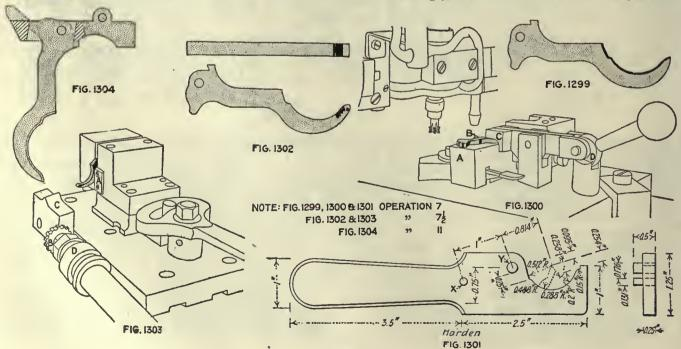
OPERATION J. FILING AND GENERAL CORNERING Number of Operators—One. Description of Operation—General filing and cornering. Apparatus and Equipment Used—File. Production—125 per hr.
