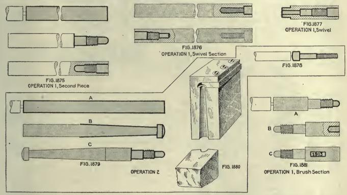
Holding Devices—Work held in draw-in chuck. Tool-Holding Devices—Turret of machine. Cutting Tools—Trimming, box tool, threading die and cutoff. Number of Cuts—Three. Cut Data—1200 r.p.m.; %-in. feed. Coolant—Cutting oil, ¼-in. stream. Average Life of Tool Between Grindings—400 pieces. Gages—Ring, thread and length. Production—50 pieces per hr. OPERATION 2. SLOTTING
