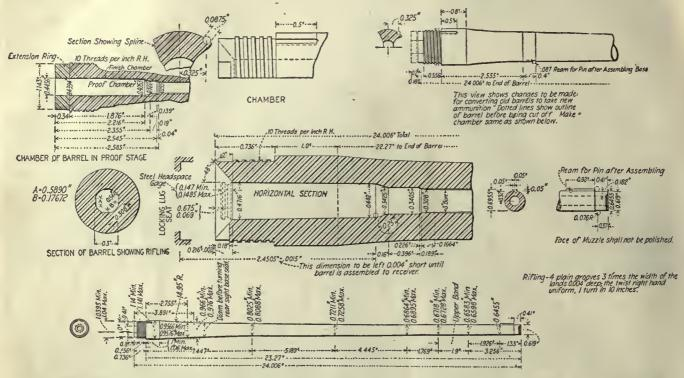
FIG. 9. SECTIONS OF SPRINGFIELD MODEL 1903 RIFLE BARREL, SHOWING WORKING LIMITS AND DIMENSIONS
