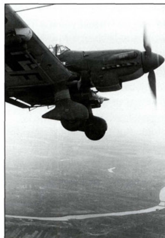
High above a sizeable Russian town (which is presumably in German hands – note the intact bridge!), an aircraft of II./StG 1 sets off on another mission. The machine is clearly carrying 50-kg (110-lb) bomb containers underwing, but closer inspection also reveals that the ventral bomb is fitted with a sturdy Dinortstab , making this one of the few known photographs of such a weapon
