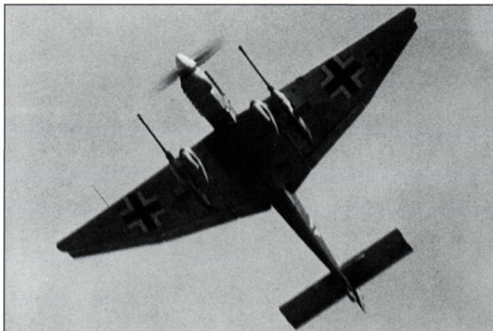
The unmistakable silhouette of another newcomer to the front early in 1943 – the 37 mm cannon-armed Ju 87G tank-buster. As feared from the air as the Tiger was on the ground, the 'Gustav' would remain a potent tank-killer right up until the end of the war
