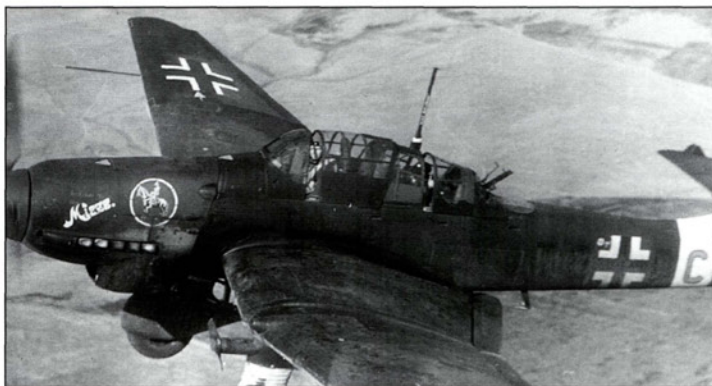
Mieze ('Pussycat') – aka aircraft 'T6+DC' of the Gruppenstab II./StG 2 – also carries additional side-armour on that partially opened canopy
