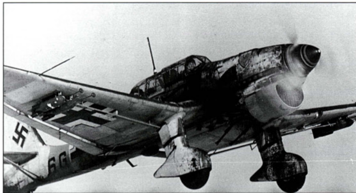
A 'Berta' of II./StG 1 labours for height. Although the ventral bomb release yoke swings empty, all four 50-kg (110 lb) underwing bombs – complete with percussion fuse rods and tail screamers – are still in situ
