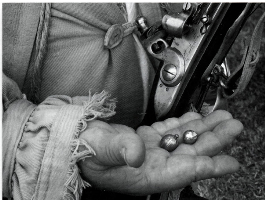
Full-caliber ball was the standard military ammunition, and today standard military ammunition is still traditionally called "ball." Note that the molding necks have not been trimmed from these balls. The brass device immediately above the large screw on the musket is a modern safety device to prevent burning bystanders with the flash from the musket pan. (Author)
